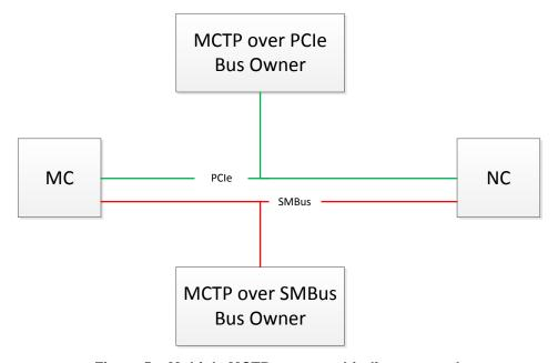
Figure 5 – Multiple MCTP transport bindings example
